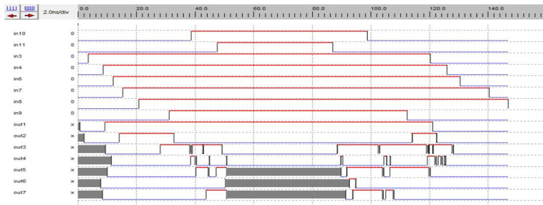
Figure 8: Circuit level Simulation Result 4\*4 Array Multiplier using GDI in Digital Schematic tool
