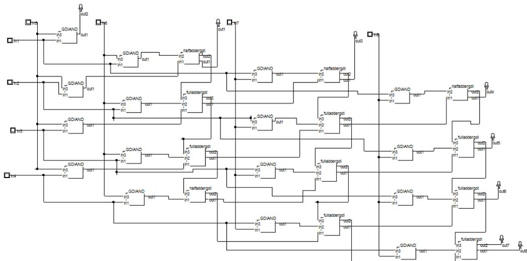
Figure 3: 4\*4 array multiplier using GDI cell
