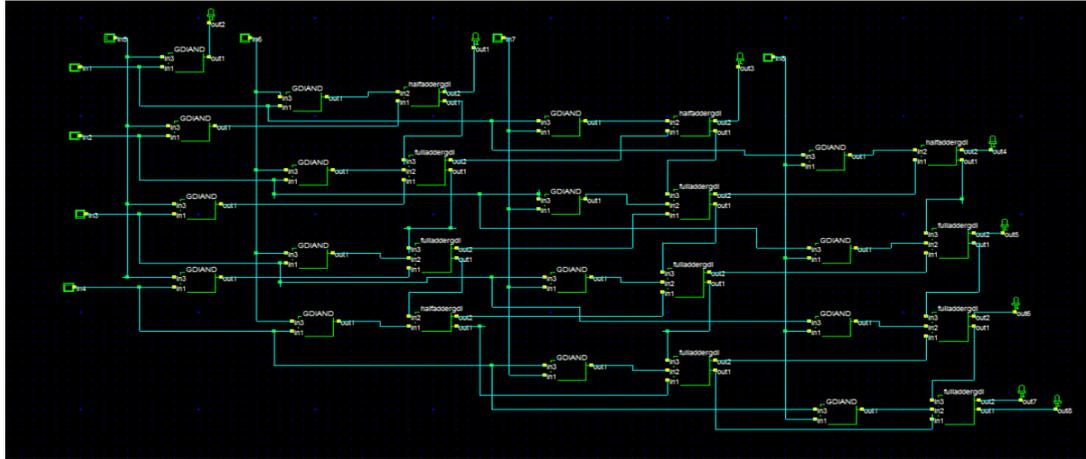
Figure 7: Schematic of 4\*4 GDI Array Multiplier using Digital Schematic tool
