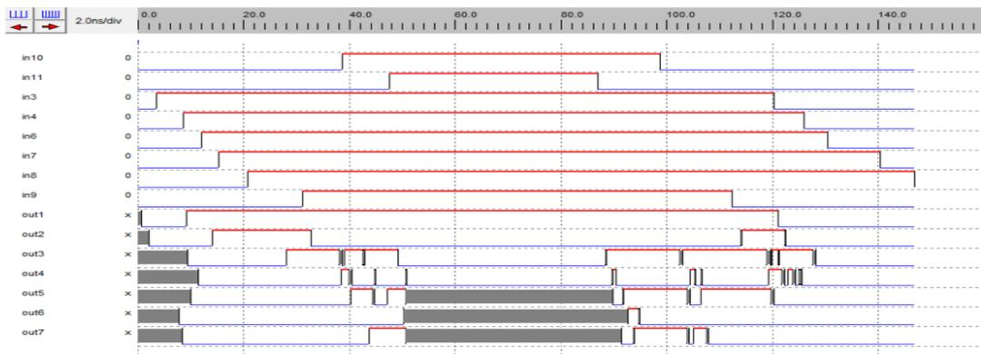
Figure 5: Circuit level Simulation Result of 4\*4 Array Multiplier using CMOS in Digital Schematic tool
