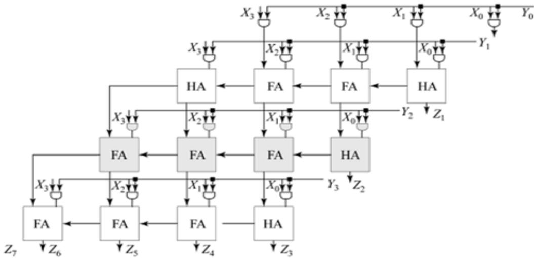
Figure 2: Block diagram of 4\*4 Array Multiplier
