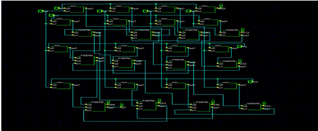
Figure 4: Schematic of CMOS 4\*4 Array Multiplier using Digital Schematic tool
