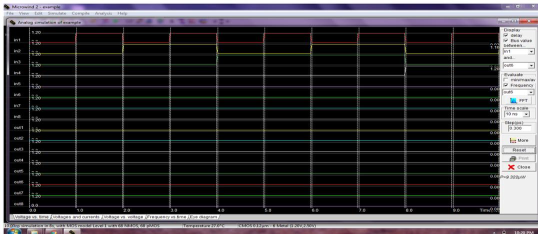
Figure 9: layout Level Simulation result of 4\*4 Array Multiplier using GDI in microwind tool
