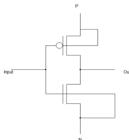
Figure 1: Circuit Diagram of GDI Cell
